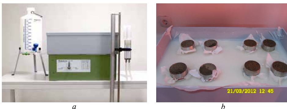
Fig. 2 – Experimental setup used to determine the suction curve: a – experimental setup; b – analysed samples.
