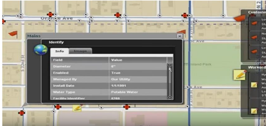
Fig. 4 – The parameters of the distribution system of the system of water supply.
