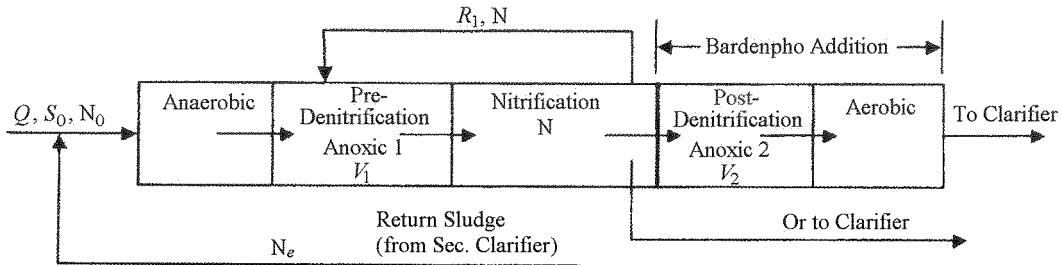
Fig. 3.– Pre-denitrification and post-denitrification schemes in biological phosphorus removal system.
