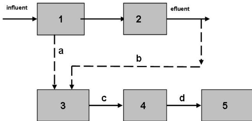
(1)- mechanical step; (2)- biological step; (3)- sludge mineralization tank ; (4)- = sludge dewatering ; (5) – final sludge deposit (a) – primarily sludge; (b) –biological sludge; (c)- digested sludge mineralized sludge (d) – dry sludge for agriculture. In particular, we are interested in chemical characteristics related to the substances content in fertilizers (N, P, K), in heavy metals and the biological characteristics with reference to the content of pathogenic agents of sewage sludge.
