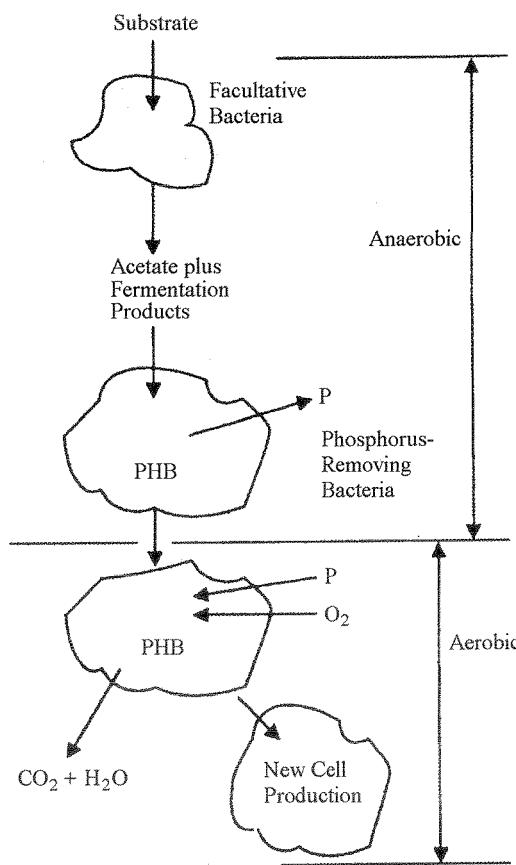
Fig. 2.- Schematic of biological phosphorus removal mechanism.
