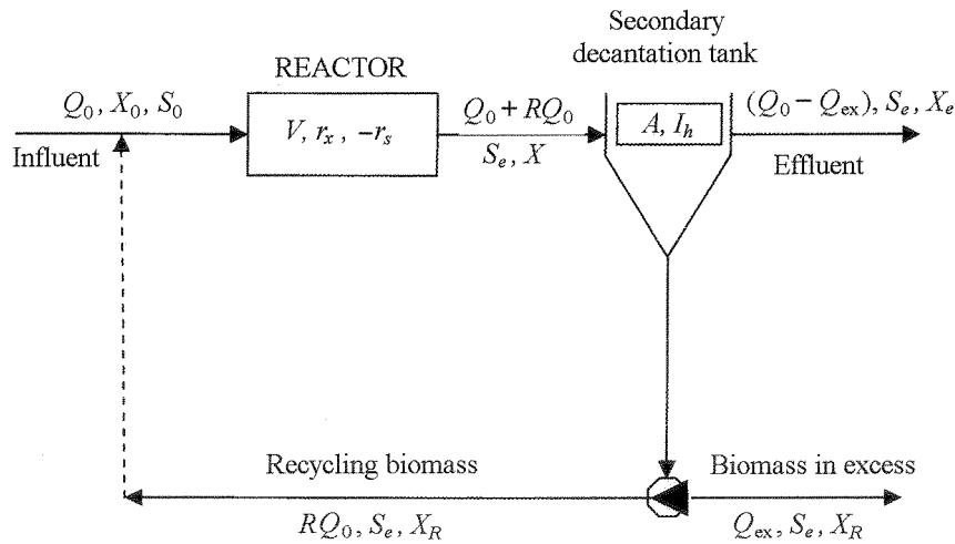
Fig. 1.– The technological diagram with a CM (compact missing) reactor and biomass recirculation (the activated sludge).
