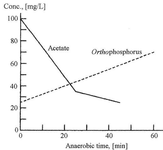
Fig. 1.– Acetate assimilation and phosphorus release *vs.* anaerobic time.
