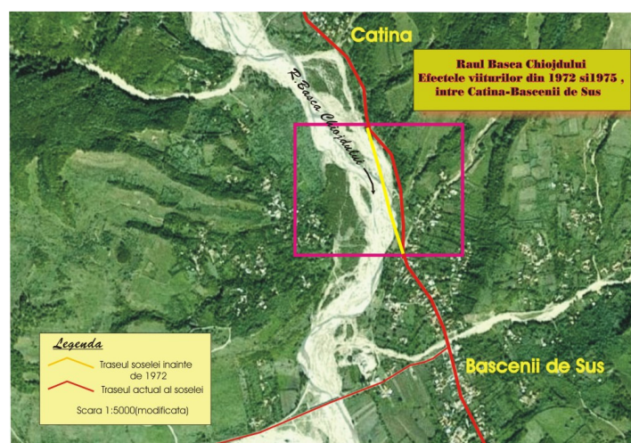
Fig. 2 – County road segment between Bâscenii de sus and Cătina destroyed by floods in 1972.
