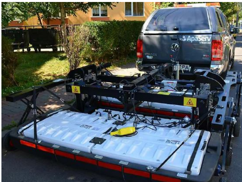
Fig. 1 – The equipment uses electromagnetic radio waves to investigate.
