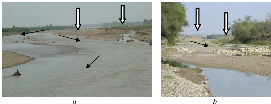
Fig. 4 – Anthropic risk factor – ballasts in the morphological modification of the river bed of Moldova: a – anthropic modification of the river flow paths; b – partial blocking of the flow through the right arm of the river in the research area through ballast deposits.
