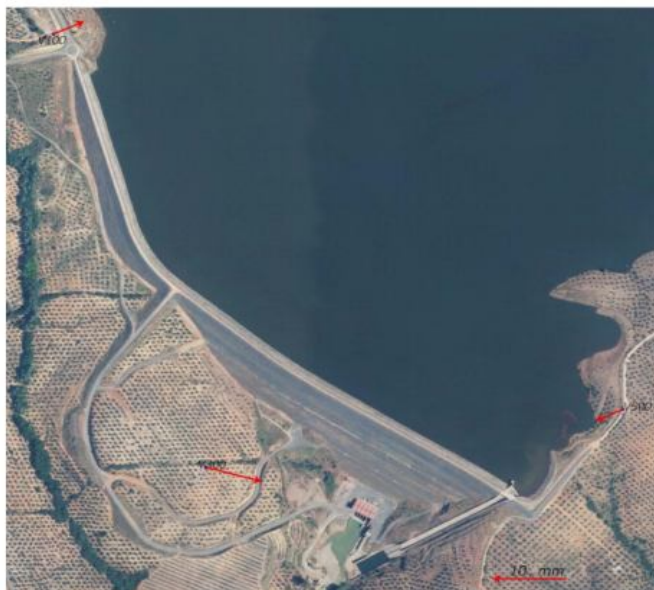
Fig. 6 – The horizontal displacements estimated for V100, V300, V500 Pillars as part of the monitoring of Arenoso dam (Acosta, 2018).
