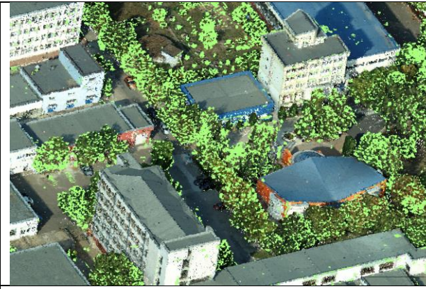
Detail integrated point cloud Phantom4+LiDAR (green)
