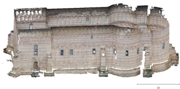
Figure 11. The dense point cloud obtained using the S1 system
