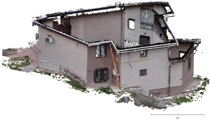
Figure 17. The dense point cloud obtained using the S2 system
