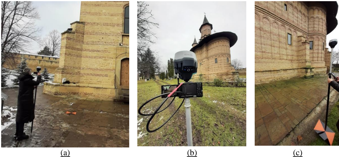
Figure 6. Acquiring images with the S1 system
